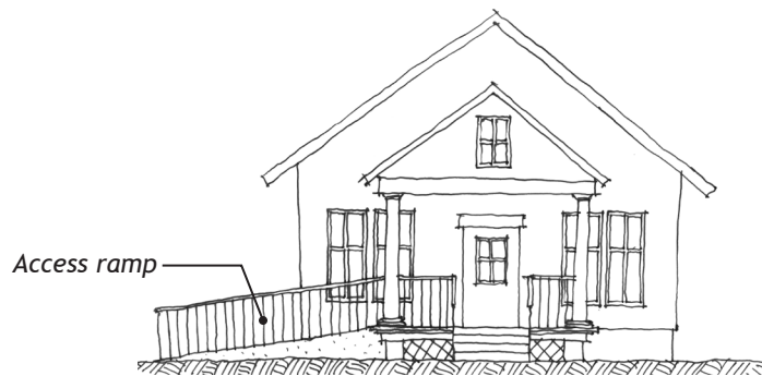
Example of a sensitive access ramp design that approaches from the side of the house.
