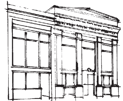
The addition is subordinate to the original building with simplified features that reflect, but do not duplicate, the historic building.
